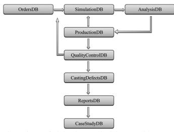
Fig. 1. Diagram of relations between SimulationDB modules
