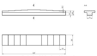
Fig. 2. Pictorial drawing of the sample
