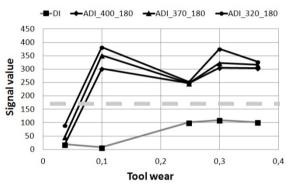
Fig. 6. Signal of acoustic emission –Ae mod. in the 2<sup>nd</sup> second of cutting for different DI samples
