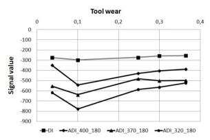
Fig. 5. Signal of acoustic emission –Ae min. for different DI samples
