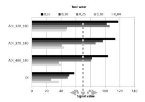
Fig. 3. Signal of cutting force -Fz in the 2<sup>nd</sup> second of cutting for different DI samples
