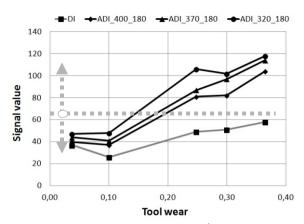
Fig. 4. Signal of cutting force -Fz in the 2<sup>nd</sup> second of cutting for different DI samples
