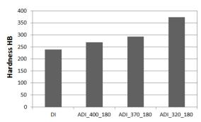
Fig. 9. Hardness of the tested DI and ADI samples
