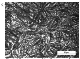
Fig. 1. Microstructure of ductile iron samples; a) DI, b) ADI 400\_180, c) ADI 370\_180, d) ADI 320\_180
