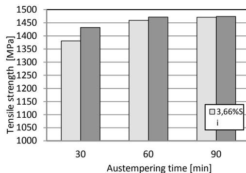
Fig. 2. The mean values of tensile strength of ADI iron obtained for different austempering time
