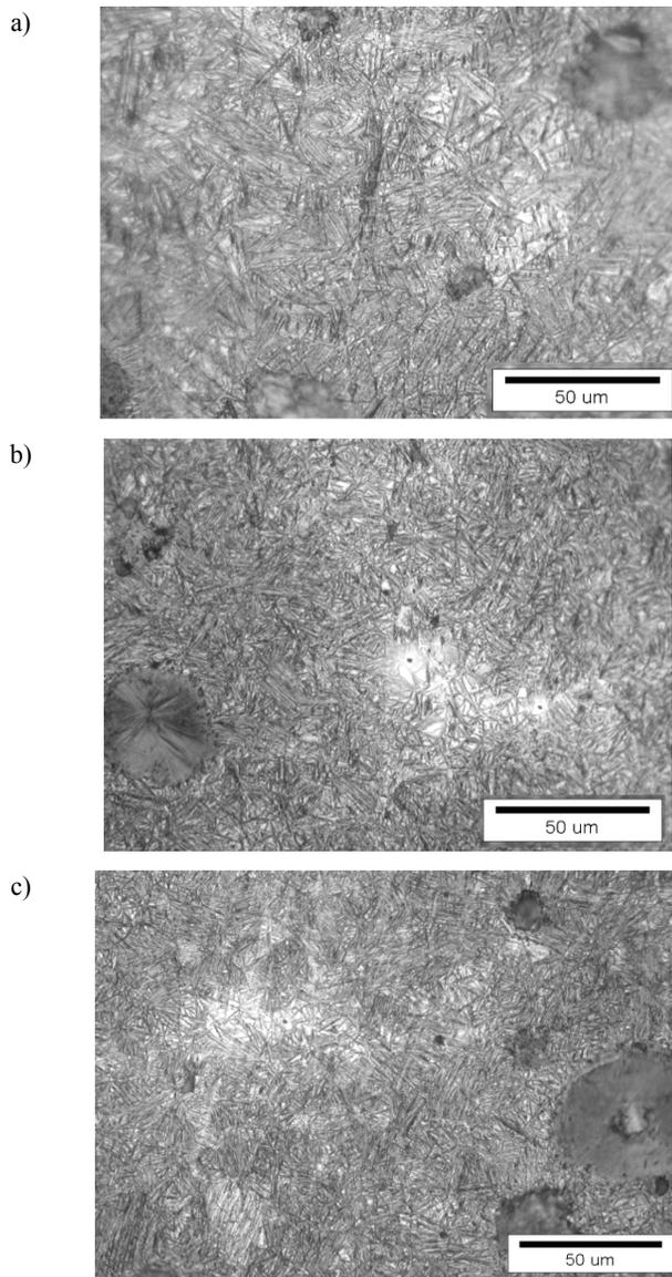
Fig. 5. The microstructure of ADI with containing 3,66% Si after austempering: a – 30, b - 60 and c - 90 minutes (x500)
