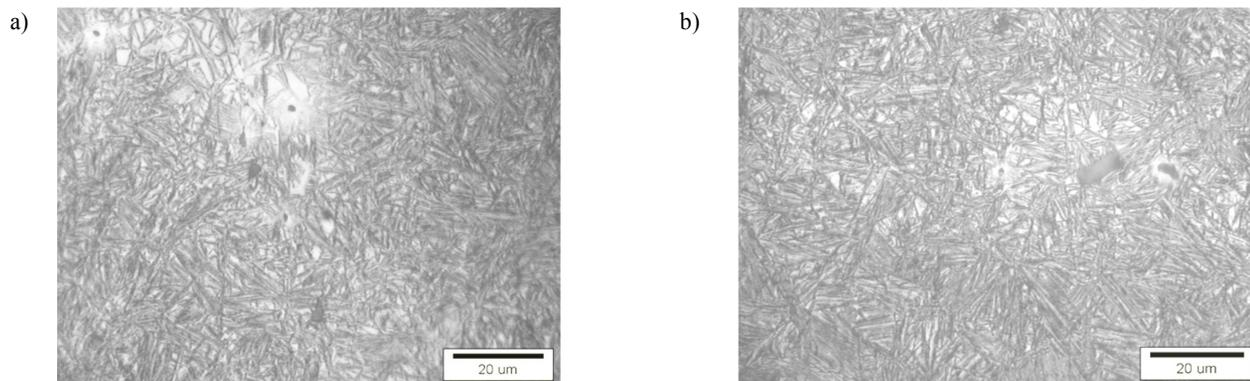
Fig. 7. The microstructure of ADI austempered 60 min. at the temperature 300°C containing: a - 3,66% Si and b - 3,80%Si observed at magnification x1000
