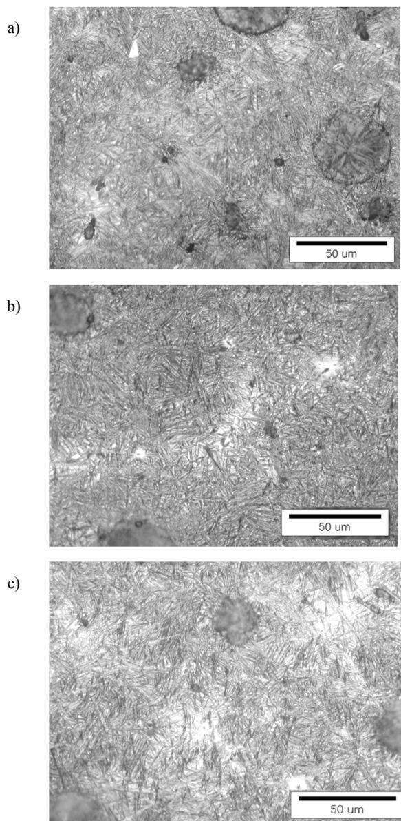
Fig. 6. The microstructure of ADI with containing 3,80% Si after austempering: a – 30, b - 60 and c - 90 minutes (x500)
