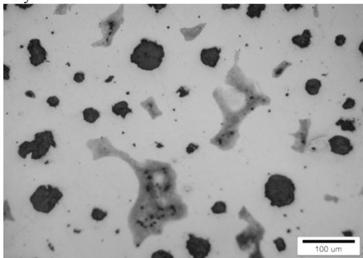
Fig. 4. The microstructure of as cast ductile iron
