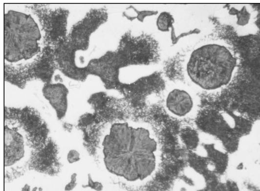
Fig. 5. Microstructure of cast iron containing 3.77% Al (melt No. 6); etched with Nital, magn. 300×
