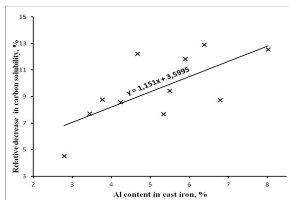
Fig. 2. The influence of aluminium content in cast iron on the decrease in carbon solubility in the alloy
