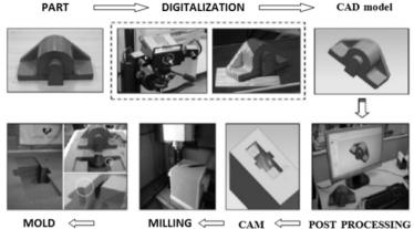
Fig. 1. Process of obtaining a mold cavity by using the method of RE and Patternless process
