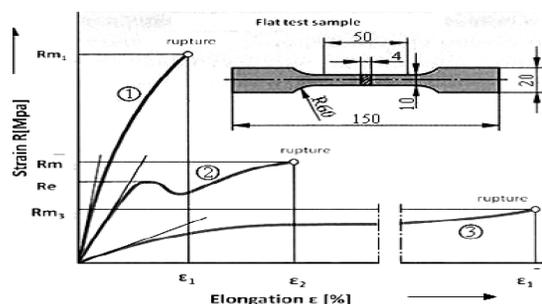
Fig. 2. Diagrams tensile test different types of plastics
