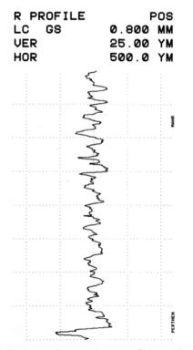
Fig. 5. Casting surface roughness profilogram from Fig. 1
