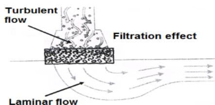
Fig. 1. An example of filtration process, the filtration cake formation and calming of the flow [5]
