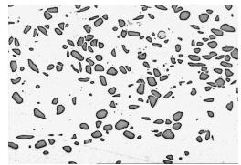
Fig. 3. Arrangement of SiC particles i composite matrix (AlSi11/10 vol.% SiC, experiment no. 10.7)
