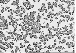
Fig. 4. Arrangement of SiC particles in composite matrix (AlSi11/20 vol.% SiC, experiment no. 20.7)
