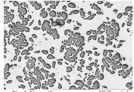
Fig. 5. Non uniform arrangement of SiC particles in composite matrix (AlSi11/20 vol.% SiC, experiment no. 20.3)
