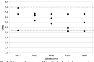
Fig. 7. Distances between carbides (l) after hardening, tempering, soft annealing and as-cast sample
