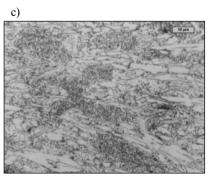
Fig. 5. Metallographic microstructure of Beta2 sample after hardening in temperature 950°C – a), tempering – b), and soft annealing – c), magnification 1000x
