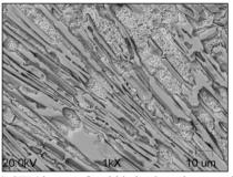
Fig. 4. SEM image of carbide in chromium cast iron, Beta sample (as-cast), magnification 1000x
