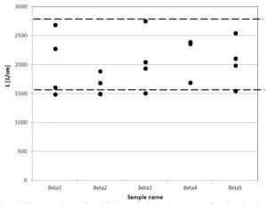
Fig. 6. The number of carbides precipitations (L) after hardening, tempering, soft annealing and as-cast sample
