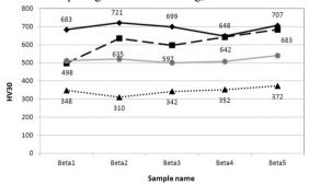
Fig. 2. The Rockwell hardness of the samples after hardening, tempering and soft annealing, and as-cast
