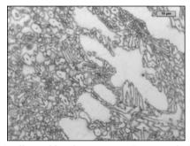
Fig. 3. Metallographic microstructure, Beta sample (as-cast), magnification 1000x
