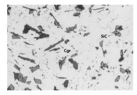
Fig. 1. Exemplary microstructure of AlMg10 + 8% SiC+2%  $C_{gr}$  composite, magn. 100×
