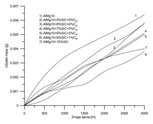
Fig. 3. Abrasive wear of the examined composites
