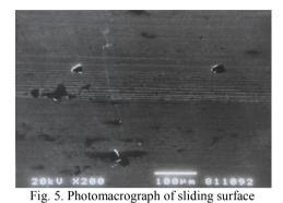
of the AlMg10 + (9% SiC and 1% C<sub>gr</sub>) composite, magn. 100×
