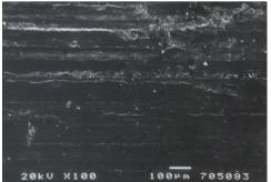
Fig. 7. Photomacrograph of sliding surface of the AlMg10 + (7% SiC and 3%  $C_{gr}$ ) composite, magn. 100×
