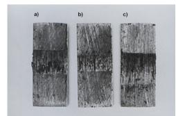
Fig. 4. Exemplary wear tracks for the examined composites: a) AlMg10+5% SiC+5% C<sub>gr</sub> composite, b)AlMg10+9% SiC+1% C<sub>gr</sub> composite, c) AlMg10 alloy
