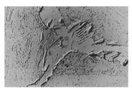
Fig. 7. Micrograph of cast iron,  $t_A = 1020^{\circ}C$ ,  $t_w = 820^{\circ}C$ ,  $\tau_w = 2$ min, TEM, microscopic magnification 5000x
