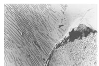
Fig. 4. Micrograph of cast iron,  $t_A$ =900°C,  $t_w$ =760°C,  $\tau_w$ =4 min, TEM, microscopic magnification 3400x
