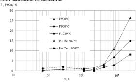
Fig. 13. Content of ferrite (F) and pearlite (P) in relation to isothermal holding time at the temperature of 820°C
