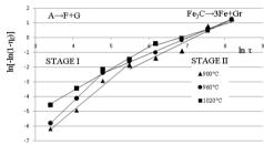
Fig. 15. Content of ferrite in relation to isothermal holding time
