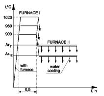
Fig. 2. Diagram of the cast iron heat treatment
