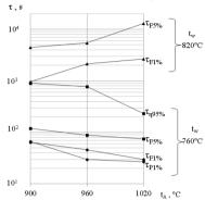
Fig. 16. Time required for a specific phase of transformation in function of austenitizing temperature
