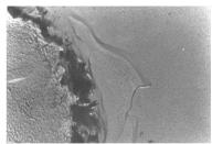
Fig. 3. Micrograph of cast iron,  $t_A=900^{\circ}\text{C}$ ,  $t_w=760^{\circ}\text{C}$ ,  $\tau_w=1\,\text{min}$ , TEM, microscopic magnification 3400x
