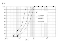
Fig. 14. Overall degree of eutectoid reaction in cast iron during isothermal holding at the temperature of 760°C
