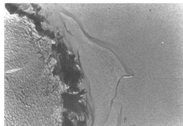
Fig. 3. Micrograph of cast iron,  $t_A=900^\circ\text{C}$ ,  $t_w=760^\circ\text{C}$ ,  $\tau_w=1$  min, TEM, microscopic magnification 3400x
