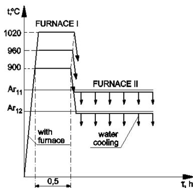
Fig. 2. Diagram of the cast iron heat treatment
