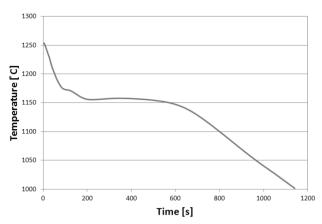
Fig. 2. Liquid metal temperature changes inside the cellulose profile
