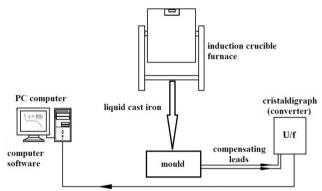
Fig. 1. Diagram of the stand for the measurement of the temperature of cast iron and profile
