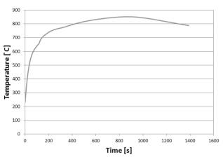
Fig. 3. Temperature changes outside the profile at the point of its surface contact with the mould material
