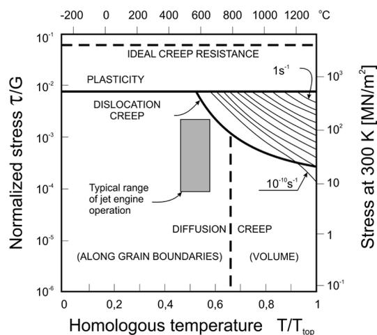
Fig. 1. Map of deformation mechanism of Mar-M200 alloy, grain size 10mm [11]
