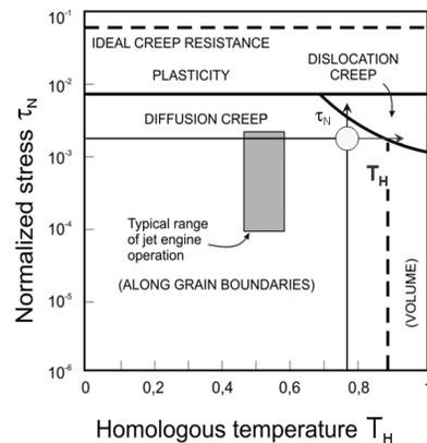
Fig. 6. A map deformation mechanisms of superalloy MAR-200 for a grain size of 0.1 mm (according to M. F. Ashby [13]). A figure schematically indicated what is the direction of the influence of increased normalized stress  $\tau_N = \tau/G$  and homologous temperature ( $T_H = T/T_{top}$ ) in the creep test on the change of creep mechanism from a diffusion creep to dislocation one
