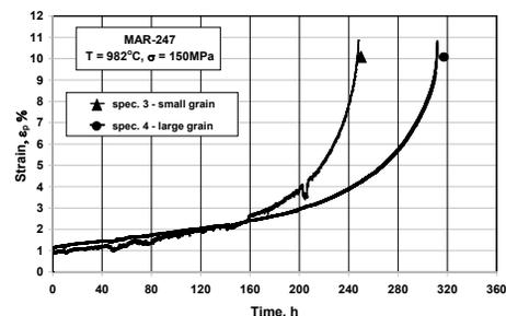
Fig. 3. Creep characteristics of nickel superalloy MAR-247 under the conditions of the I variant
