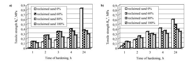
Fig. 1. Influence of the hardening time on the tensile strength,  $R_m^u$  of the moulding sand of the composition: high-silica sand 0 – 100 parts by mass, reclaim 0 – 100 parts by mass, GEOPOL binder 2.0 parts by mass, hardener – 14% of the binder amount: a) SA72, b) KR72
