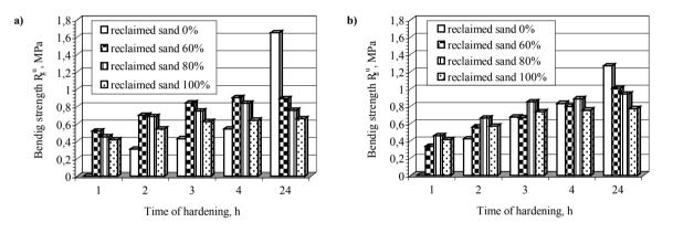
Fig. 2. Influence of the hardening time on the bending strength,  $R_g^u$  of the moulding sand of the composition: high-silica sand 0 – 100 parts by mass, reclaim 0 – 100 parts by mass, GEOPOL binder 2.0 parts by mass, hardener – 14% of the binder amount: a) SA72, b) KR72
