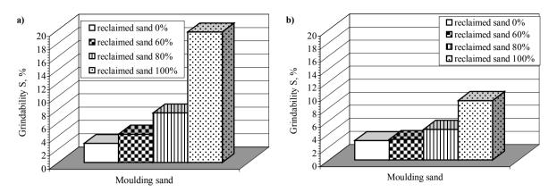
Fig. 4. Influence of the reclaim addition on the grindability, S of the moulding sands of the following composition: high-silica sand 0 - 100 parts by mass, reclaim 0 - 100 parts by mass, GEOPOL binder 2.0 parts by mass, hardener - 14% of the binder amount: a) SA72, b) KR72
