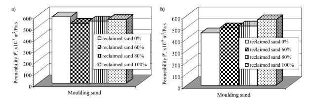
Fig. 3. Influence of the reclaim addition on the permeability,  $P^{u}$ , of the moulding sand of the following composition: high-silica sand 0 – 100 parts by mass, reclaim 0 – 100 parts by mass, GEOPOL binder 2.0 parts by mass, hardener – 14% of the binder amount: a) SA72, b) KR72
