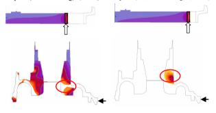
c) piston speed during filling of mould cavity – 10 m/s
