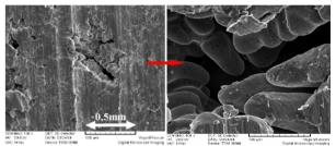
Fig. 1. SEM micrographs of shrinkage porosity (Al-Si-Cu), The dendrite tips are visible what confirms the shrinkage origin of
