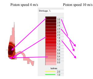
Fig. 9. Shrinkage porosity for two piston speed
