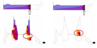
Fig. 8. Simulation results of air entrapment phenomena corresponding to chosen stages of piston positions in shot sleeve. a – in shot sleeve from beginning to final piston position, b – two chosen stages (70 step and 89 step) connecting the piston position with air entrapment map inside of casting (for different piston speed)
