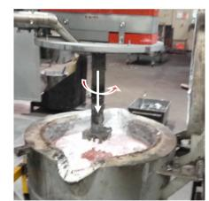
Fig. 4. Test stands used for testing: a) apparatus DTA-Cristaldigraph, DI-MK and FMA, b) rotor (refining process with argon)
