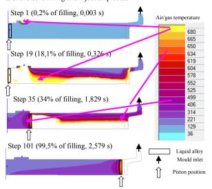
b. piston speed during filling of mould cavity - 4 m/s
