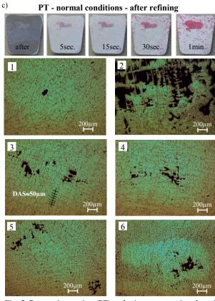
Fig. 5. Penetrating testing (PT) and microstructure in selected sites in cup casting: a) plan of both samples, b) before refining, b) after refining
