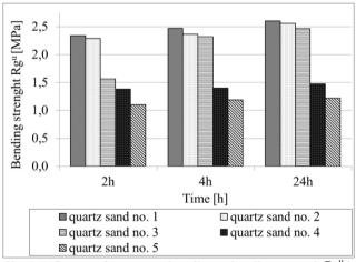
Fig. 1. Influence of quartz sand quality on bending strength R<sub>g</sub><sup>u</sup> in moulding sands with furfural resin
