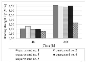
Fig. 3. Influence of quartz sand quality on bending strength  $R_g^{u}$  in moulding sands with alkyd resin
