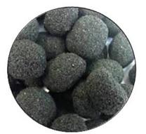
Fig. 11. Precursors – Furan molding mixture (regular shape and size)
