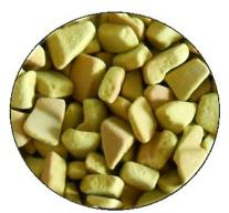
Fig. 10. Precursors - Croning process (irregular shape and size)
