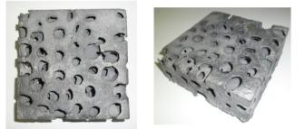
Fig. 6. Casting (cast iron with lamellar graphite) - type I
