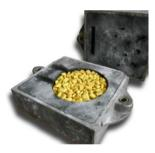
Fig. 2. Mold made from commonly used green sand
