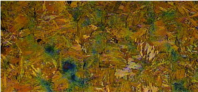
Fig. 1b. Equiaxed structure revealed within the 15-ton steel ingot
