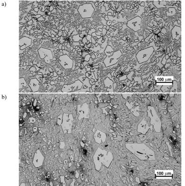
Fig. 4 Microstructure of the high Cr cast iron with 4.28 wt. % C: a – as-cast; b – after heat treatment (austenitizing at 900°C, tempering at 450°C)
