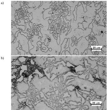
Fig. 3. Microstructure of the high Cr cast iron with 2.72 wt. % C: (a) as-cast; (b) after heat treatment (austenitizing at 900°C, tempering at 450°C)
