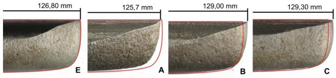
Fig. 1. The change in a length and shape of the worn hammers made from the as-cast high chromium cast irons A, B, C, and the reference hammer made from the X210Cr 12 steel (E)
