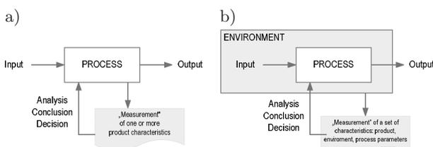
Fig. 1. a) Classical approach to the evaluation of the manufacturing process state b) Approach to the evaluation of the process state with a consideration of the process and its environment
