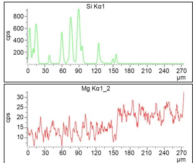
Fig. 13. Concentration of Si and Mg along the measuring line from Fig. 12
