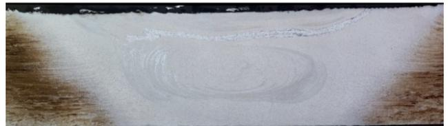
Fig. 9. Structure of FSW weld in the case of locating the rod of EN AC-43200 (A) on the retreating side. Welding parameters:  $\omega = 900 \text{ min}^{-1}$ ,  $V = 224 \text{ mm/min}$ . Triflute pin. Etching: Keller
