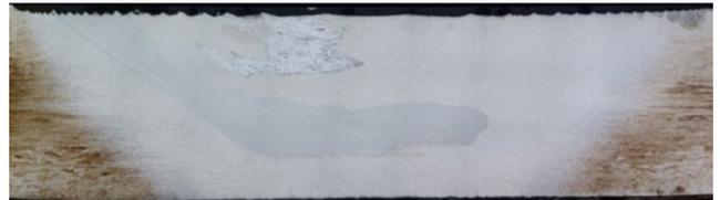
Fig. 6. Structure of FSW weld in the case of locating the rod of EN AC-43200 (A) on the advancing side. Welding parameters:  $\omega = 450 \text{ min}^{-1}$ ,  $V = 224 \text{ mm/min}$ . Triflute pin. Etching: Keller
