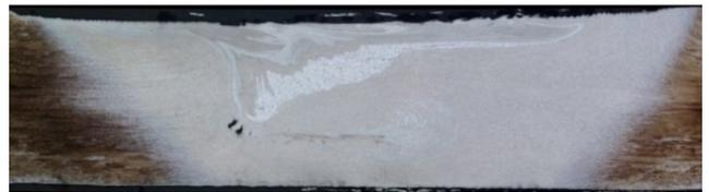
Fig. 8. Structure of FSW weld in the case of locating the rod of EN AC-43200 (A) on the advancing side. Welding parameters:  $\omega = 900 \text{ min}^{-1}$ ,  $V = 224 \text{ mm/min}$ . Triflute pin. Etching: Keller
