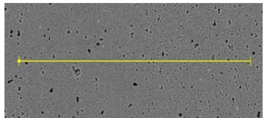
Fig. 14. Fragment of the structure from Fig. 8. Welding parameters:  $\omega = 900 \text{ min}^{-1}$ ,  $V = 224 \text{ mm/min}$ . Triflute pin. SEM-EDS chemical composition analysis was conducted along the marked line (Fig. 15)
