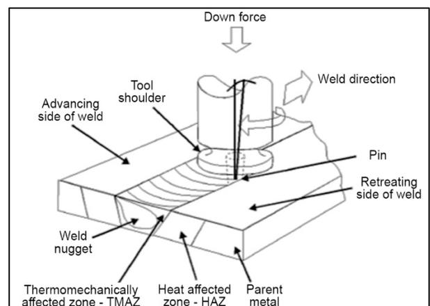
Fig. 1. The scheme of the FSW process [1]
