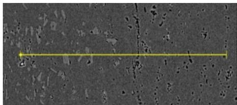
Fig. 12. Fragment of the structure from Fig. 6. The boundary between EN AC-43200 alloy (from the left side) and EN AW-6082 alloy (from the right side). Welding parameters:  $\omega = 450 \text{ min}^{-1}$ ,  $V = 224 \text{ mm/min}$ . Triflute pin. SEM-EDS chemical composition analysis was conducted along the marked line (Fig. 13)
