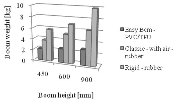
Fig. 6. Weight by different type of boom
