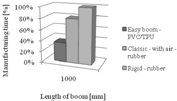
Fig. 9. Manufacturing time of boom [8]
