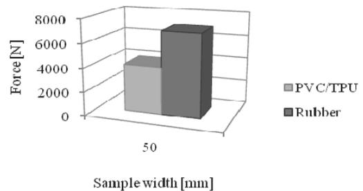
Fig. 7. Tensile strength of PVC/TPU and rubber for oil boom on 50 mm width sample
