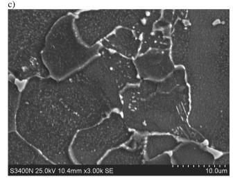
Fig. 2. Carbides morphology in 13HMF steel, tube  $\emptyset$  273 × 32 mm. Observations performed at metallographical samples SEM, detector: a) BSE, b), c) SE
