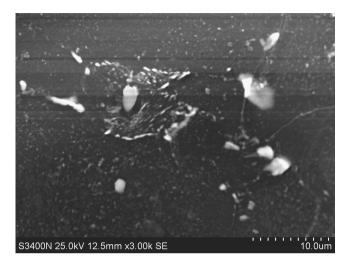
Fig. 4. Carbides morphology in 13HMF steel microstructure, tube  $\emptyset$  273 × 32 mm. Extraction replica, SEM, detector SE
