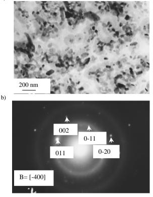
Fig. 5. a) Dispersed MC precipitates, TEM image b) Diffraction pattern of MC precipitates
