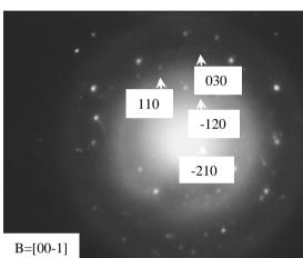
Fig. 6. a) Dispersed  $M_2C$  precipitates, TEM image b) Diffraction patern of  $M_2C$  precipitates
