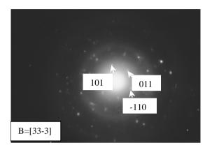
Fig. 8. Diffraction pattern of particle shown by arrow in Fig. 7,  $M_{23}C_6\, \mbox{precipitate}$
