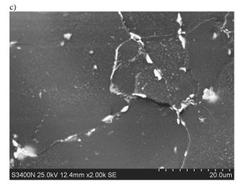
Fig. 3. Carbides morphology in 13HMF steel, tube  $\emptyset$ 273×32 mm. Extraction replica, SEM, detector SE
