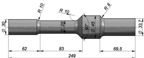
Fig. 1. Shape and dimensions of the lever preform [9]
