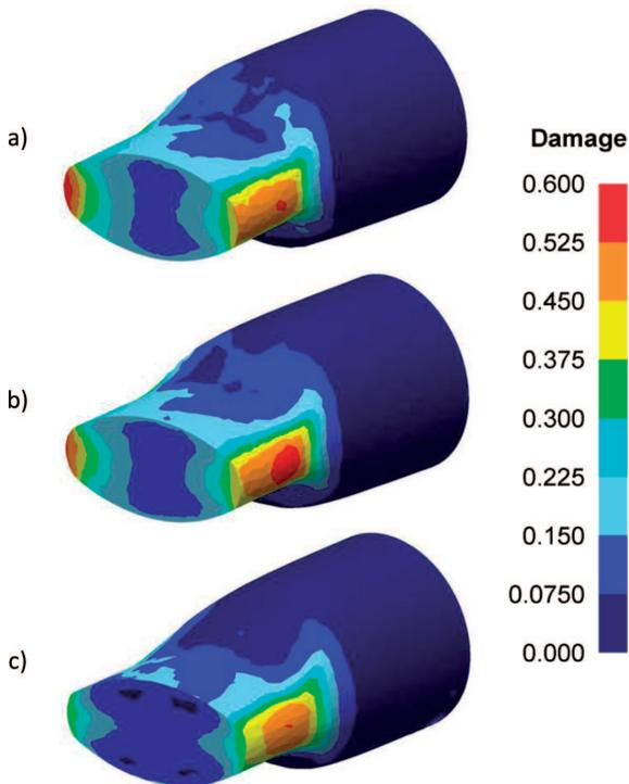
Fig. 6. Distribution of Cockcroft-Latham integral value: a) segment with radius  $R = 10$  mm, b)  $R = 20$  mm, c) segment with gradually increasing reduction ratio
