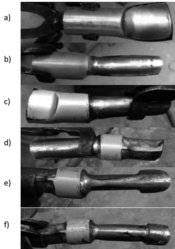
Fig. 12. Subsequent roll passes during rolling of the preform from billet with diameter  $\varnothing 42$  mm: a) oval - I, b) circle - I, c) oval - II, d) circle - II, e) oval - III, f) circle - III
