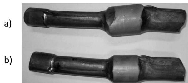
Fig. 13. Forgings from magnesium alloy AZ31 rolled in the forge rolling process: from billet with diameter  $\varnothing 45$  mm, b) from billet with diameter  $\varnothing 42$  mm
