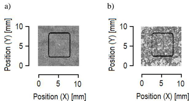
Fig. 12. Laser-ultrasonic 2-D C-scan with assumed sound depth: a) 1.5 mm, b) over 3 mm.
