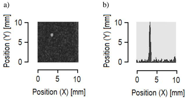
Fig. 10. Laser-ultrasonic 2-D C-scan (a) with an assumed sound depth of 1.5 mm and profile (b).
