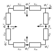
Fig. 1. Equivalent circuit diagram of a grounding grid.
