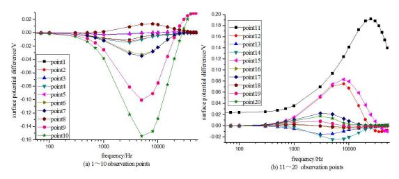
Fig. 3. Potential amplitude differences between observation points 1 ~20.
