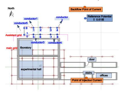
Fig. 5. Observation points of a factual grounding grid.
