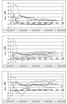
Fig. 6. Influence of learning data vector length on the result of prediction of corrections for the UTC(PL) using the regression method for time series: a) ts1, b) ts2 with regression coefficients  $a_1$  i  $a_0$ , c) ts2 with regression coefficient  $a_1$ .
