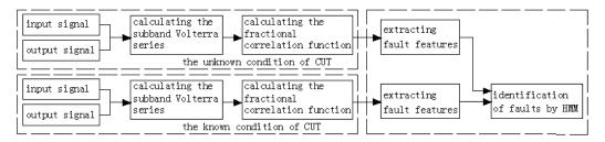
Fig.1. The block diagram of the proposed method.
