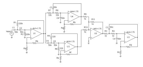
Fig. 3. Simulation 1- The band-pass filter circuit.
