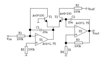
Fig. 10. Logarithm amplitude circuit in simulation 2.
