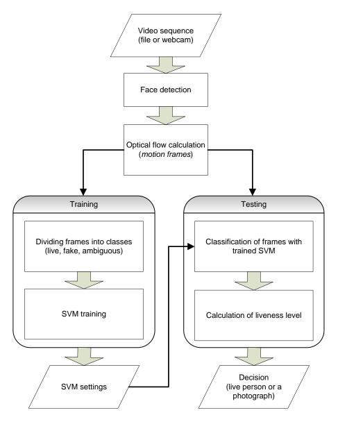
Fig. 1. The simplified block diagram of a liveness detection method.
