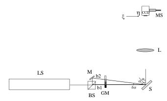
Fig. 1. Experimental set-up. LS, laser beam; BS, Beam splitter; M, mirror; GM, gradual mirror;  $\alpha_i$ , incidence angle;  $\alpha_o$ , observation angle; S sample; L, lens; MS, micrometer screw; CCD camera.
