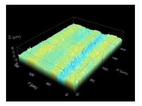
Fig. 3. Titanium surface. (a) 2D diagram. The distinct colors correspond to different microscopic heights. (b) 3D representation. Observe the anisotropy.
