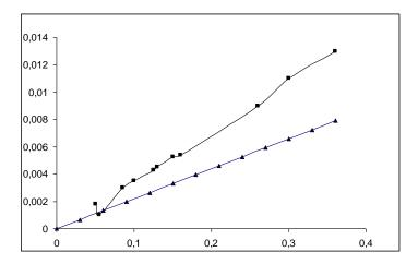
Fig. 5. The lower straight line shows the theoretical curve for the shift of the speckle pattern when the angle of the incident illumination beams is changed (Eq. (4)). The x-axis corresponds to the focal length f and the y-axis the speckle field displacement on the CCD camera. The upper curve corresponds to the actual displacements for the lenses used in the experiments.
