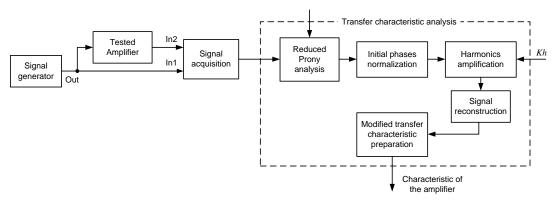
Fig. 3. Method of analysis of the tested system's transfer function.
