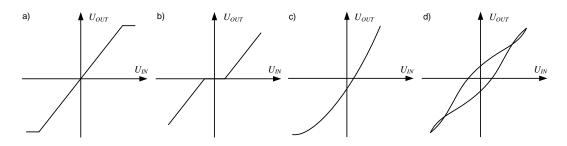
Fig. 1. Types of transfer function of signal amplifiers.
