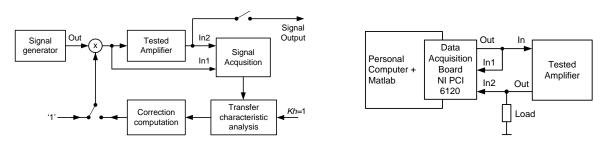
Fig. 4. Method of generating a corrected amplified signal.
