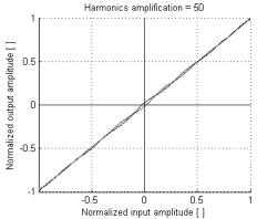
Fig. 8. Corrected transfer function of *amplifier I* with amplified harmonics.
