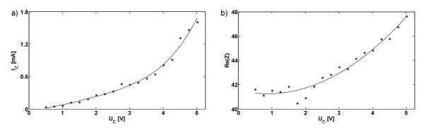
Fig. 10. The changes of current a) and equivalent series resistance b) as a function of operating point of a supercapacitor of 0.22 F capacity and 5.5 V nominal voltage obtained by the AC method at a frequency of 1kHz.
