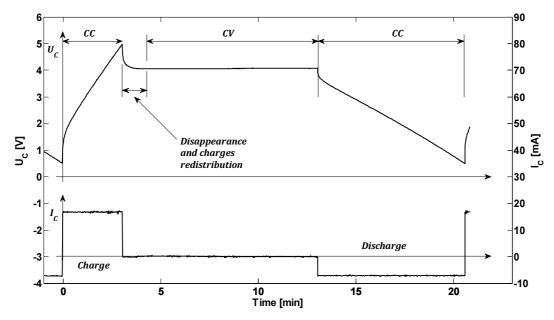
Fig. 9. The current and voltage curve during tests of a 1 F and 5.5 V nominal voltage supercapacitor.
