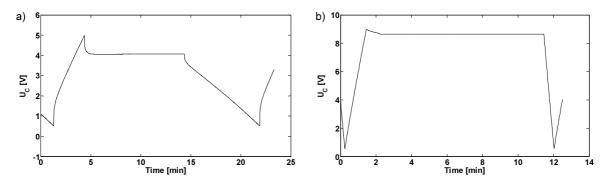
Fig. 2. Charge/discharge cycle of two kinds of capacitors: a) 1 F supercapacitor, b) 3300  $\mu$ F typical electrolytic capacitor.
