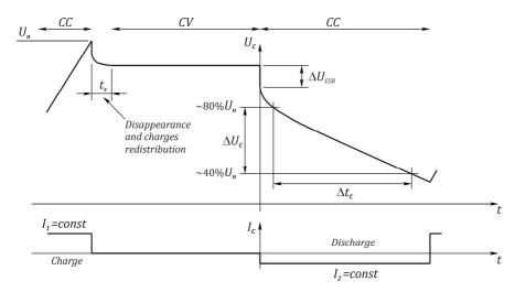
Fig. 5. The method of determination of the values of supercapacitor parameters with constant current CC and constant voltage CV.
