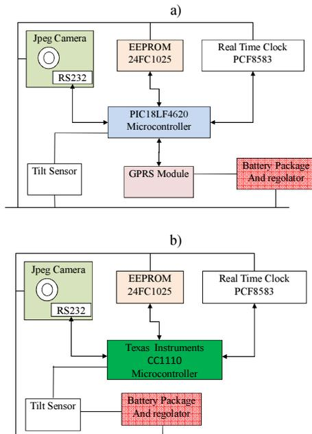
Fig. 2. Block diagram of visual sensor:
