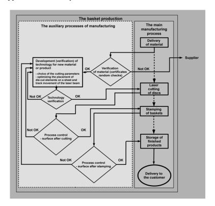
Fig. 9. Scheme of the support and control systems.
