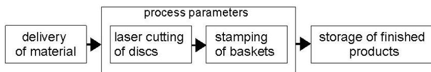
Fig. 2. The technological process of the basket production steps.
