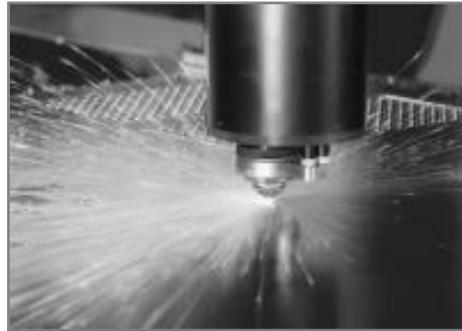
Fig. 3. Cutting bores with a laser cutter
