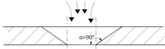
Fig. 8. Proposed shape of the waste basket bores.
