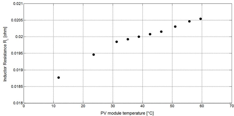
Fig. 6. Inductor resistance dependence on PV module temperature.
