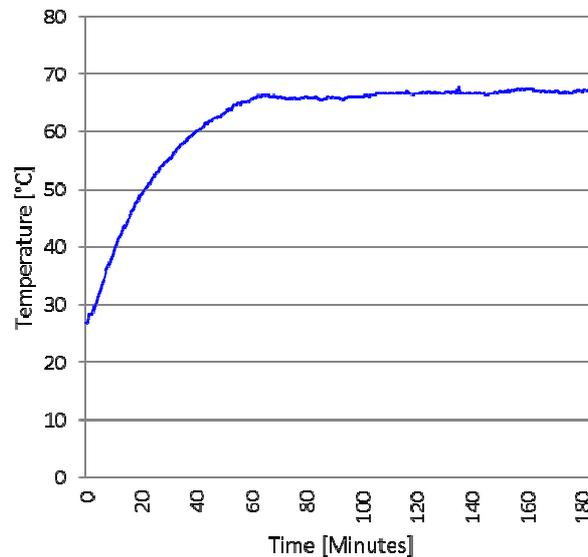
Fig. 10. MOSFET temperature vs time after design upgrade.
