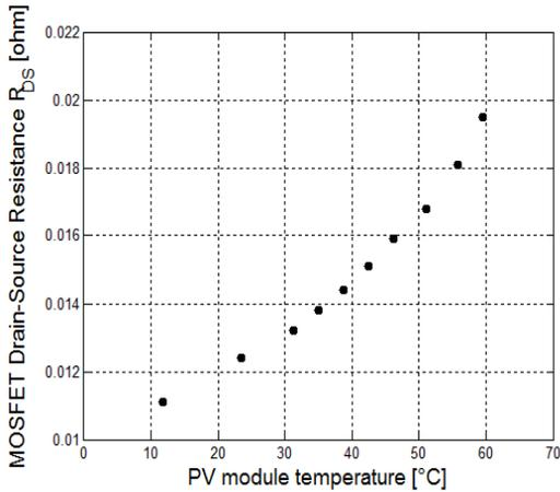
Fig. 4. MOSFET Drain-Source Resistance vs PV module temperature.
