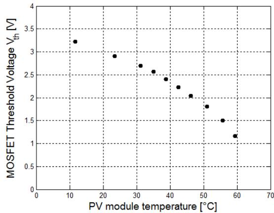
Fig. 5. MOSFET Threshold Voltage vs PV module temperature.
