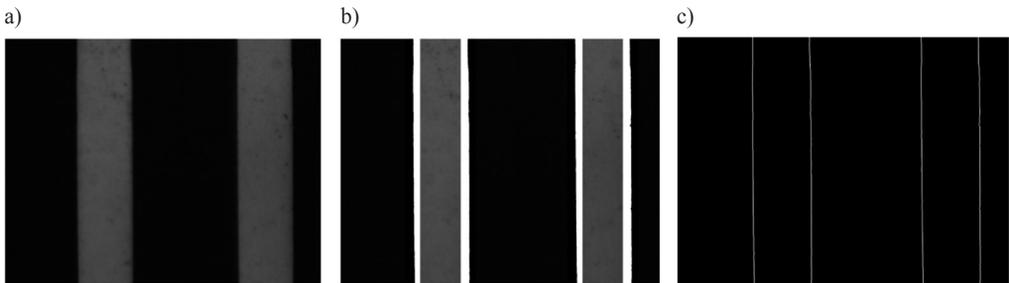
Fig.3. ROI extraction and local segmentation: a) several edges in an image; b) local segmentation in ROI; c) the detected stripe edges.
