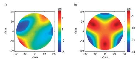
Fig. 3. a) Deformation of a double-sided polished silicon wafer; b) the GID of a silicon wafer obtained using the three-point-support inverting method.
