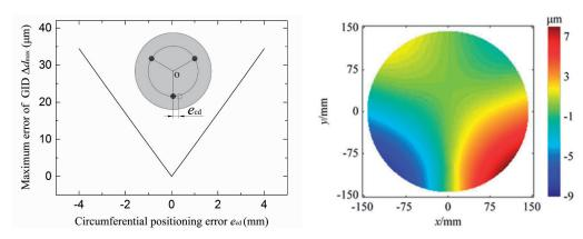
Fig. 13. The relation between  $\Delta d_{\text{max}}$  and  $e_{\text{cd}}$ .
