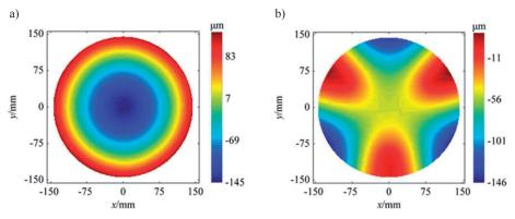
Fig. 8. a) Deformation of the ground silicon wafer, b) the GID of the wafer obtained using the three-point-support inverting method.
