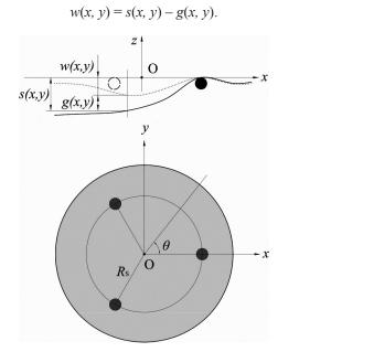
Fig. 1. An illustration of a silicon wafer supported by three balls.
