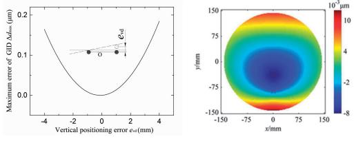
Fig. 15. The relation between  $\Delta d_{\text{max}}$  and  $e_{\text{vd}}$ .
