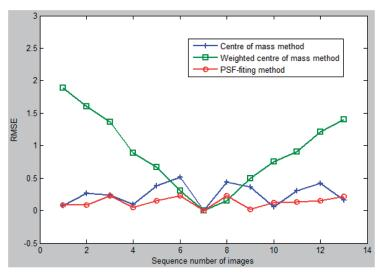
Fig. 9. The root mean squared error of centroid determination for three different methods: centre of mass, weighted centre of mass and PSF-fitting.
