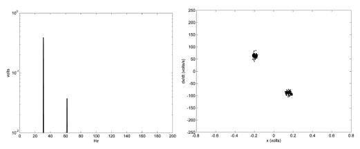
Fig. 5. The motion at  $\Omega = 61.9$  Hz for  $a_b = 4$  g.
