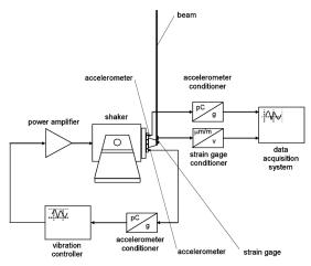
Fig. 1. The experimental setup.
