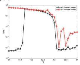
Fig. 4. The frequency-response curve of the third mode  $\omega_3$  for  $a_b = 4$  g.
