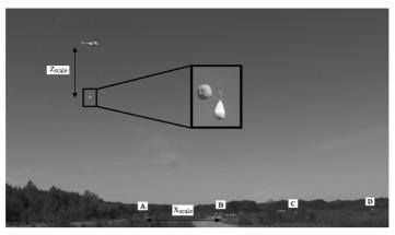
Fig. 2. Arrangement of the experimental setup during helicopter's flight. The helicopter carrying a water capsule hanging on a rope is visible on the left. The capsule is equipped with a stabilizing parachute.
