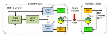
Fig. 5. A simplified block diagram of the TFTS-2 system.
