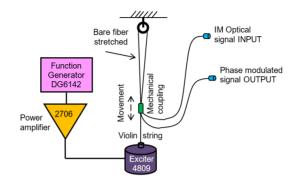
Fig. 2. A block diagram of the fibre stretcher.
