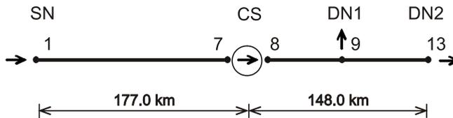
Fig. 1. Structure of the gas transportation system, SN-sending node. CS-compressor station, DN1, DN2-delivery nodes
