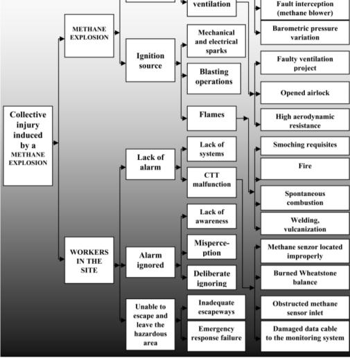
Fig. 1. Reduced Root – Cause tree for the undesired event "Collective injury induced by a methane explosion"
