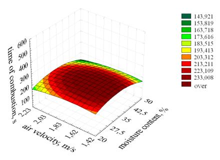
Fig. 10. The influence of suspension moistness and air flow velocity on the fuel combustion time in a fluidized bed;  $T = 850^{\circ}C$
