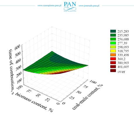
Fig. 7. The influence biomass and coal-mule content in suspension on the fuel combustion time in a fluidized bed;  $T = 850^{\circ}C$
