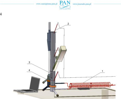
Fig. 4. The research stand for fuel combustion in a stream of air and in a circulating fluidized bed (without insulation); 1 – gas heater, 2 – thermocouple Ni-CrNi, 3 – visualization pane, 4 – inert material pouring out place of fluidized bed material
