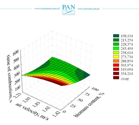
Fig. 5. The influence of air flow velocity and the biomass content in suspension on the fuel combustion time in a fluidized bed;  $T = 850^{\circ}C$
