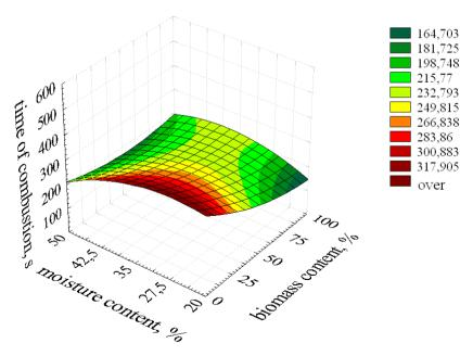
Fig. 6. The influence of suspension moistness and biomass content in suspension on the fuel combustion time in a fluidized bed;  $T = 850^{\circ}C$
