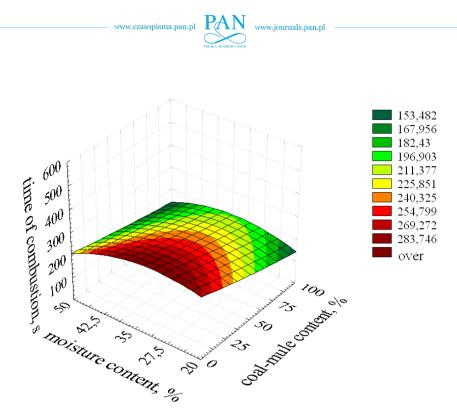
Fig. 9. The influence of suspension moistness and coal-mule content in suspension on the fuel combustion time in a fluidized bed; T = 850°C
