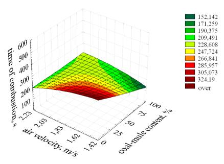
Fig. 8. The influence of air flow velocity and coal-mule content of suspension on the fuel combustion time in a fluidized bed;  $T = 850^{\circ}C$
