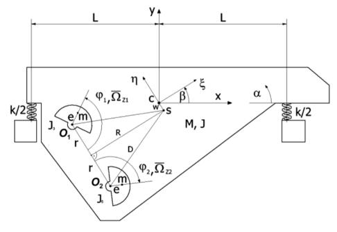
Fig. 1. Two-vibrator over-resonance vibratory machine calculation model
