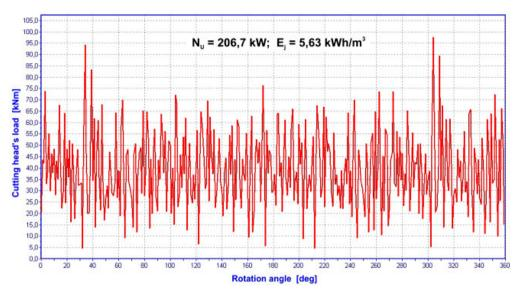
Fig. 3. The curve of the moment of load forces on the cutting head shaft while cutting the rock with the compressive strength of  $R_c = 80 \text{ MPa}$
