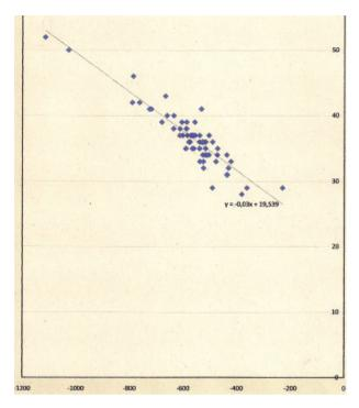
Fig. 3. Dependece of temperature on depth from the measurements of maximum temperature in mine forbores. Calculated values: Temperature gradient  $G_{100} = 3.0^{\circ}/100$  m. Correlation coef. -0.905
