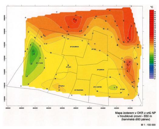
Fig. 2. Example of a map of isothermal lines in the Karviná subbasin of OKR from NP bores in the depth of -650 m. Crosses indicate the location of boreholes
