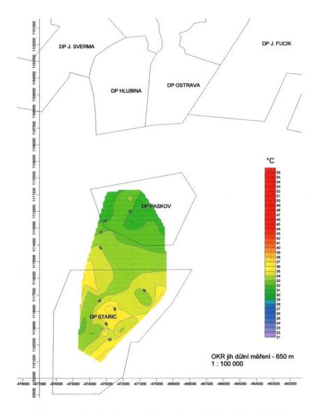
Fig. 6. Map of isothermal curves of the southern subbasin in the depth of -650 m
