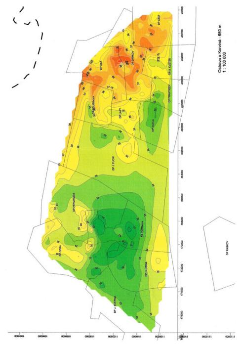
Fig. 5. Map of isothermal curves of the Karviná and Ostrava subbasin in the depth of -650 m
